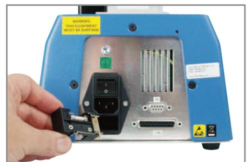
To change the operating voltage, remove the fuse cartridge, turn it over and re-fit
