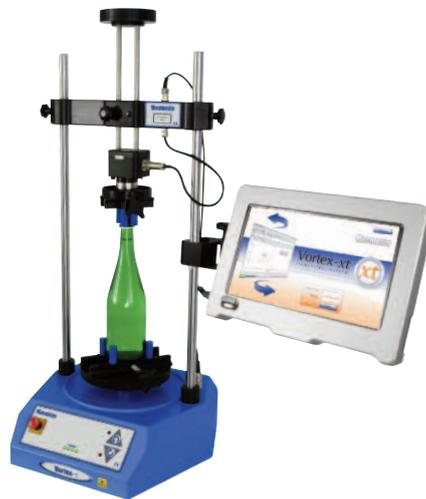
Slide the crosshead onto the two support columns and tighten both securing thumbscrews. Different height samples can be accommodated by moving the complete crosshead up and down. Additional adjustment is available by moving the top-load carrier. If a top-load is to be used, the securing knob is generally left un-done during measurement so the carrier can slide up and down. If a top-load test is not to be used, securely tighten the locking knob after adjusting to the height required.
