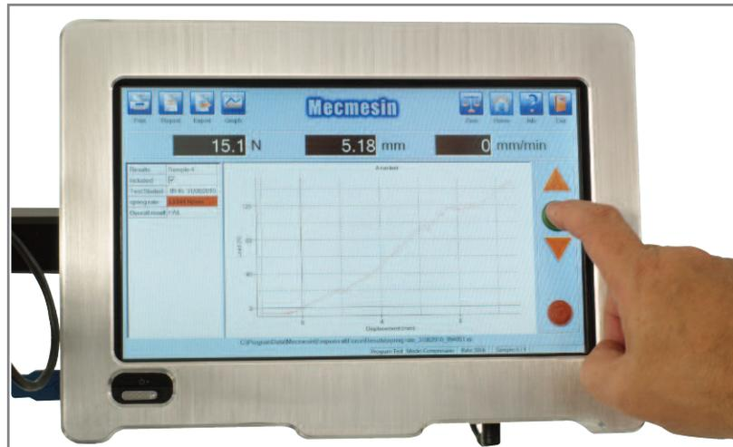
Start the Quick Test by pressing the green Start button
