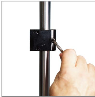
Attach the collar to one of the Vortex-xt supports using the allen key supplied
