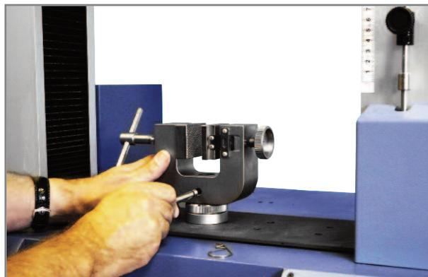
The QC system for rapid attachment of grips shown on a MultiTest 25-xt
