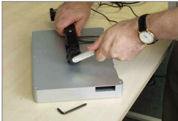
Use the tool to remove the security collet - N.B. this has a left-hand thread
