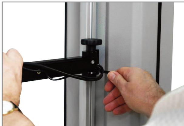
Slide the “T” shaped securing fasteners into the slot on the rear of the stand and tighten using the Torx wrench supplied
