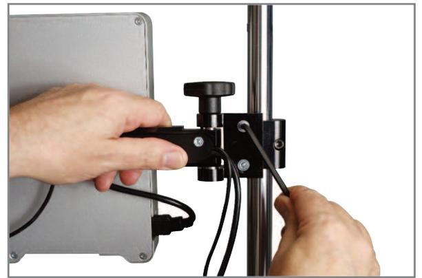
Fit the Console bracket to the collar using the Torx wrench supplied to tighten the two screws
