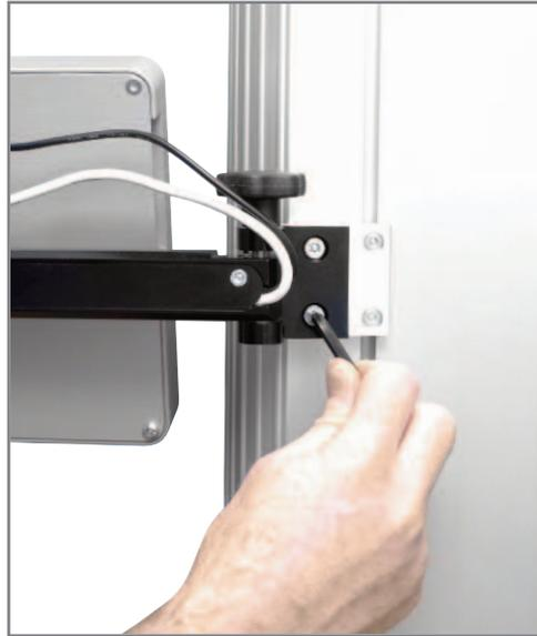
**Fitting the Console to the twin-column mounting plate**
