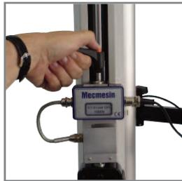
2. Tighten the securing screw using the clamp handle.
