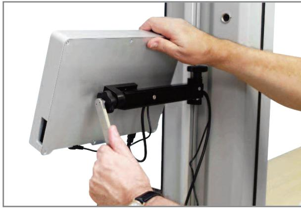
**Re-attach the Console to the bracket arm and re-fit the adjusting knob and the security collet. Tighten the security collet anti-clockwise**
