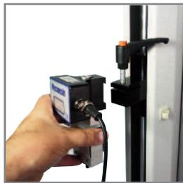
1. On single column test stands slide the loadcell (ILC) sideways onto the dovetail bracket at the front of the crosshead. The threaded stud must always be on the underside.
