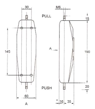
Please note that if you wish to use the gauge with a Mecmesin test stand then an additional bracket will be required. This will increase the \* dimension by 13.5mm approximately.
